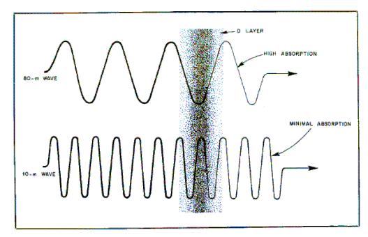
All conditions being equal, a lower frequency signal will undergo greater D-layer absorption than a higher frequency.
